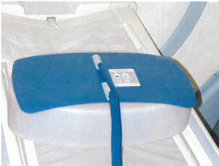
FIGURE 3. Experimental set-up used to evaluate artifacts for the Arctic Sun, Energy Transfer Pad. The Arctic Sun, Energy Transfer Pad was placed on the outside of a copper sulfate phantom to simulate its intended in vivo use. The phantom with the Arctic Sun, Energy Transfer Pad was the subjected to MRI at 3-Tesla using three different pulse sequences.
