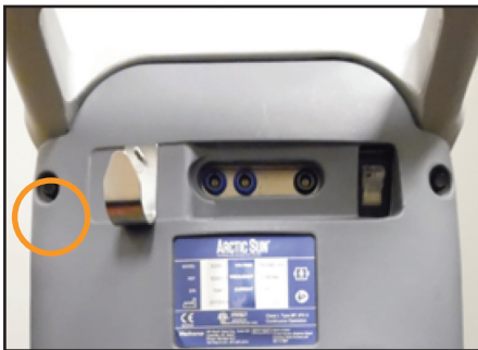
Fig. 8-72 Remove bolt (Step 1)
