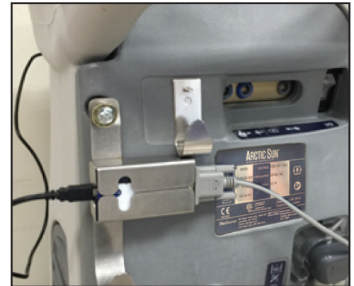
Fig. 8-74 Insert TIM and connect cables (Steps 3-5)
