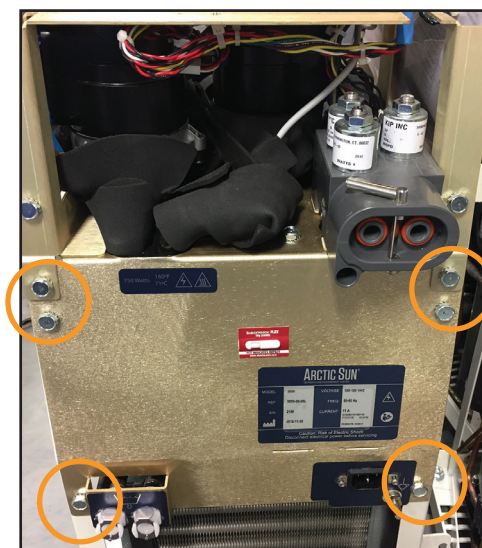
Fig. 8-36 Remove six bolts (Step 3)
