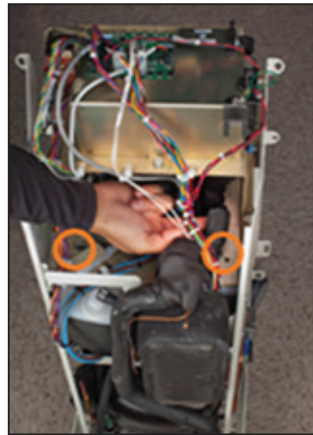
Fig. 8-17 Remove two bolts (Step 2)
